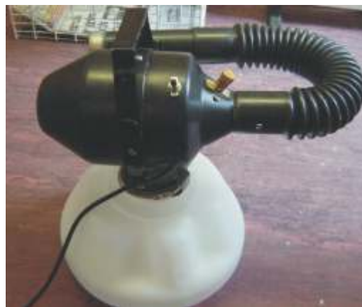
Fogger used to overspray in aviaries and poultry houses in the presence of the birds.
